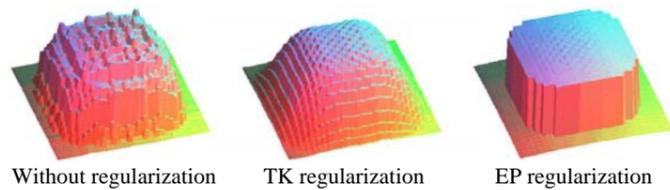
**Fig. 1. Contrast profile of a square polystyrene object**
